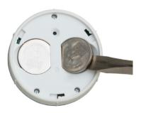
5. Insert new batteries, making sure each is snug.
